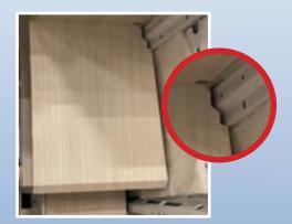
Our cabinets are custom CNC cut to duplicate the sidewall profile of the Van. This process improves the amount of usable space inside the vehicle. This gives 8% extra usable interior space.
