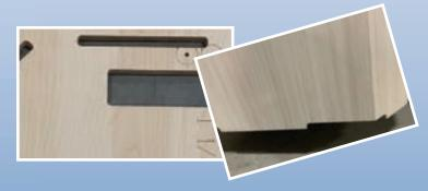
Base cabinets are precision docked into notches in the subfloor. This extra step keeps cabinets "rock solid" in place preventing fatigue from hard braking and rough road travel.
