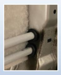
Plumbing lines that pass-through chassis steel are rubber grommeted to protect the integrity of the system and prevent future wear issues.
